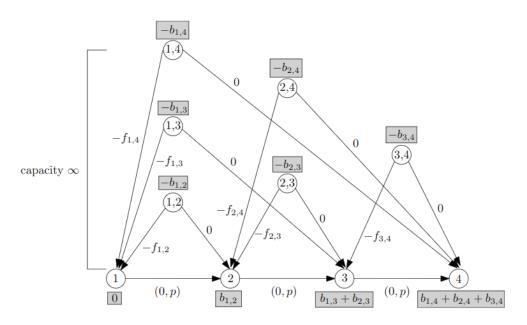
The arcs between nodes represent the path of the plane with capacity p, cost 0.
