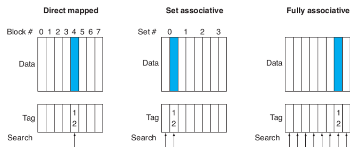
Figure 2.4 The location of a memory block whose address is 12 in a cache with eight blocks varies for direct-mapped, set-associative, and fully associative placement
